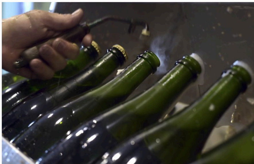
Bottles of crémant d'Alsace sparkling wine are pictured during the disgorging process, on August 12, 2016, in Steinbach, France. Photographer: PATRICK HERTZOG/AFP
